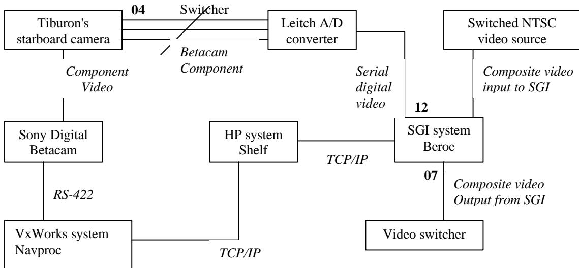
To configure vicki so that the *Snap Main* button grabs images from Tiburon's right camera video source 04 must be set to destination 12. Any other composite NTSC video source may be mapped to destination XX and the *Snap Aux* button will grab images from that source.
